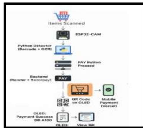
Smart Trolley System with OLED UI and QR- based Payment Integration
